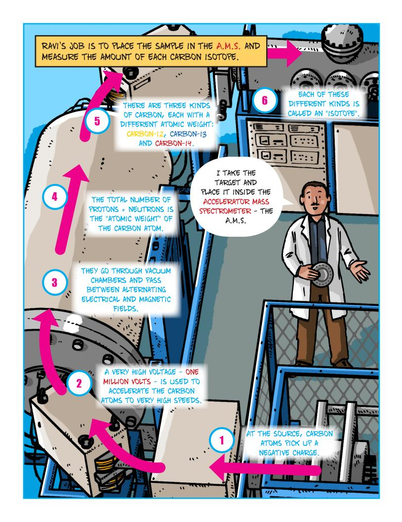
THE A.M.S. MACHINE USES ELECTRICAL AND MAGNETIC FIELDS TO SEPARATE THESE ISOTOPES.
